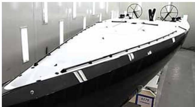
A heavily chamfered sheer adds to the modern look of the new Carkeek 47 while reducing both aero drag and structural weight
